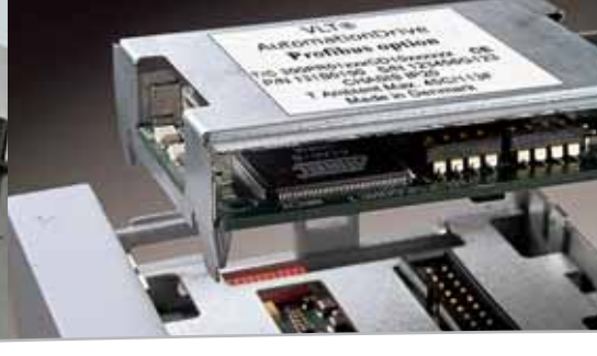
The fieldbus option ready to plug in beneath the front panel. It can be turned upside down if you'd rather have the cable on top.
